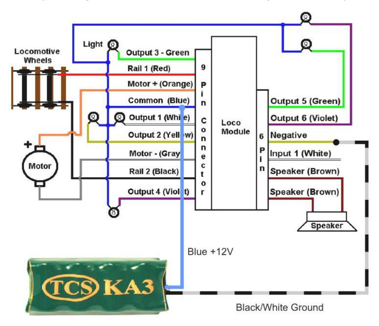
Module 9 Pin Blue (Common Wire) to KA3/4 Blue +12v Wire
